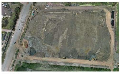
2nd Month Initial eathwork of the site required excavation of existing soil while also mixing it with specified engineered soil.
